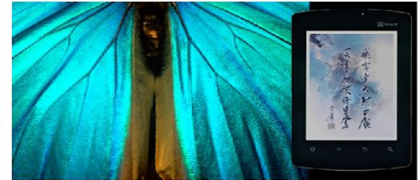
The Mirasol screen mimics the structure of butterfly wings to make e-reader and tablet displays easier to see while using less power.
